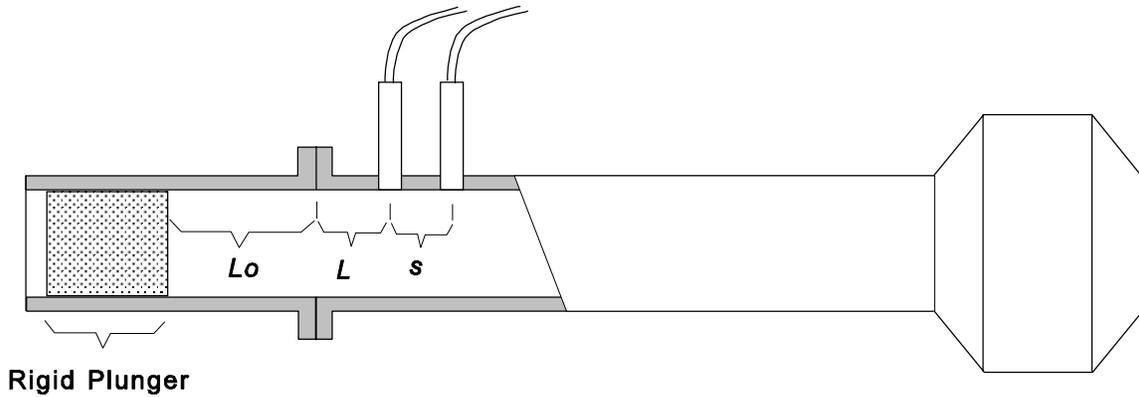
**Figure 2 Measuring the impedance of a closed tube.**
