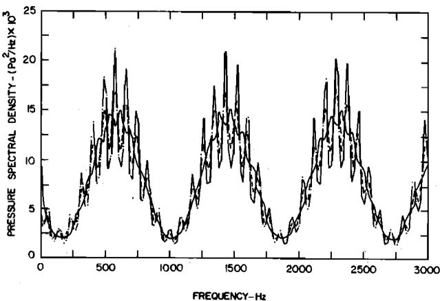
FIG. 7. Approximate calculation of the estimate  $E[\hat{S}_{pp}]$  and the true value  $S_{pp}$  of the auto-spectral density function at  $x = 0.2 \text{ m}$  from the sample for several analysis bandwidths. Broken line:  $S_{pp}$ , dashed line:  $E[\hat{S}_{pp}]$  for bandwidth = 50 Hz. Solid line:  $E[\hat{S}_{pp}]$  for bandwidth = 100 Hz.
