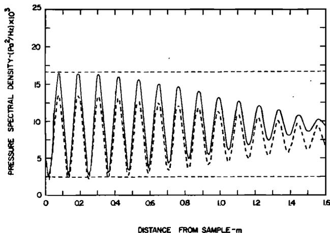
FIG. 8. Approximate and exact calculation of the auto-spectral density function estimate  $E[\hat{S}_{pp}]$  versus distance from sample at 1500 Hz for  $\Delta f=100$  Hz. Dashed line:  $S_{pp}$ ; dotted line: Exact  $E[\hat{S}_{pp}]$ ; solid line: Approximate  $E[\hat{S}_{pp}]$ .
